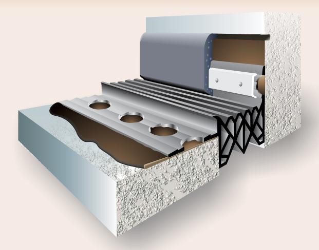
Thixotropic ambient-cured polyurethane material for expansion joint systems formulated to hold the Santoprene seal in its place.
