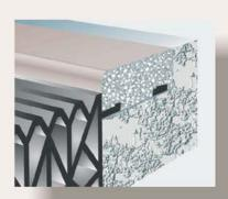
Rapid-setting ambient-cured polyurethane material compounded with a sand/aggregate mixture to form a durable nosing material for expansion joint applications
